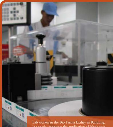
Lab worker in the Bio Farma facility in Bandung, Indonesia, monitors the application of labels with incorporated vaccine vial monitor technology. Photo by Umit Kartoglu
